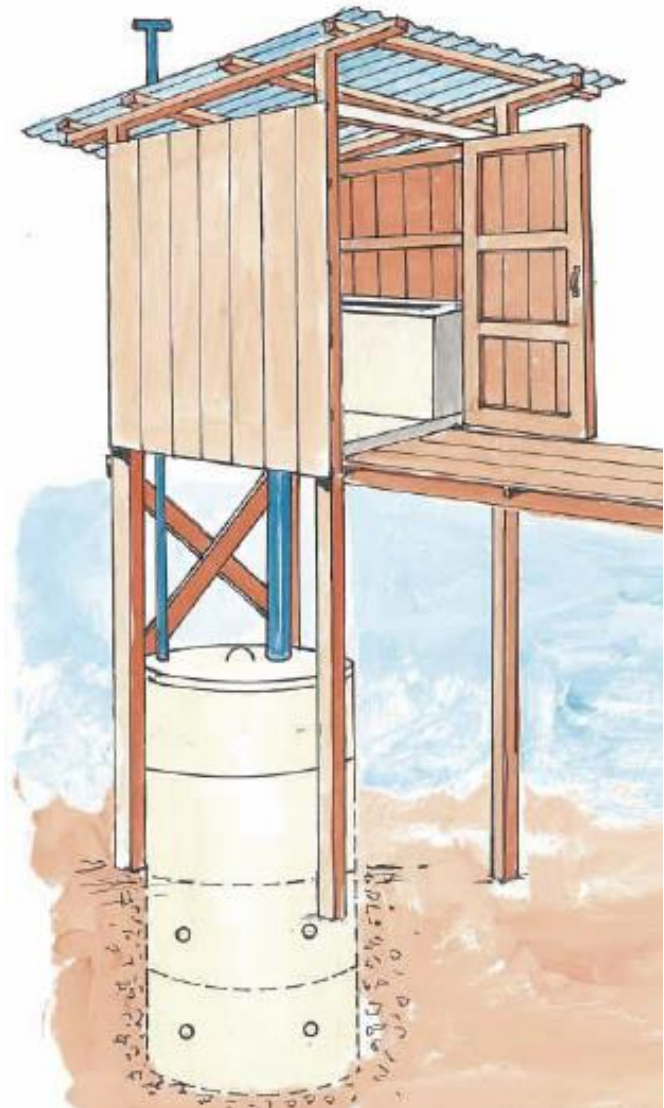
Figure 2: Raised toilet pit, Source: MRD, SNV/2011
